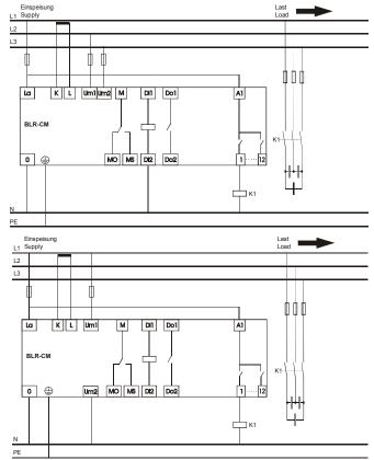
5) Remove short circuit links of the current transformer before commissioning!
